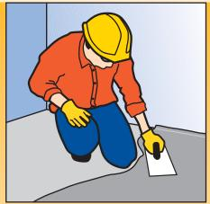
14. The 2nd and 3rd coats of Sika®-1 Screed Mortar are applied to the floor by trowel and lapped onto wall finishes.
