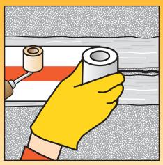
All joints should be protected by SikaDur®-Combiflex® System incorporated within the render.
