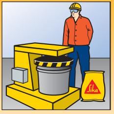
Sika®-1 pre batched Mortars must be mixed in forced action mixers using Sika®-1 gauging solution.
