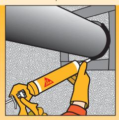
15. All service entries must be filled with Sika®-1 Waterproofing System and sealed using high performance sealants Sikaflex®-11FC+, SikaSwell® or SikaDur®-Combiflex® System.
